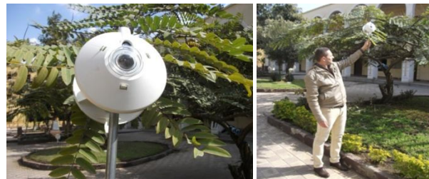
Fig 2 Albedo measurements use 2 back to back CMP21 second class high temperature pyranometer as Albedometer manufactured by Kipp and Zonen
