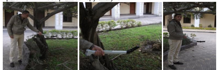
Fig 4 Using LAL2200c plant canopy analyzer in field measurements
